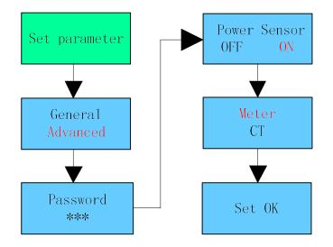
If you only want to check the load consumption function, you can choose Meter as Power sensor. CT is just only for Export Limit function.
