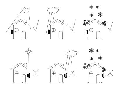
Please make sure the inverter is installed at the right place. The inverter can't install close to trunk.
