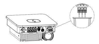
4. Insert two AC terminal block insulation partitions.
