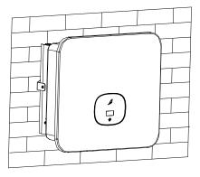
After confirming the inverter is fixed reliably, fasten one M6 safety-lock sockets head cap screws on the right or left side firmly to prevent the inverter from being lifted off the bracket.
