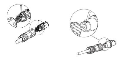
**Step 2** Push the threaded sleeve into the socket, Tighten up the cap on the terminal.
